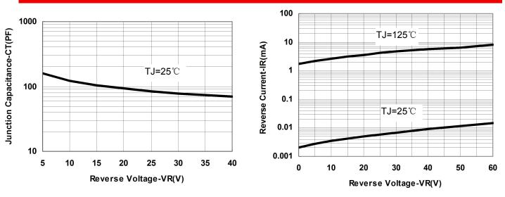
**Fig.1-Typical Junction Capacitance**
