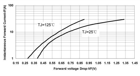
Fig.3-Typical Instantaneous Forward Voltage Characteristics
